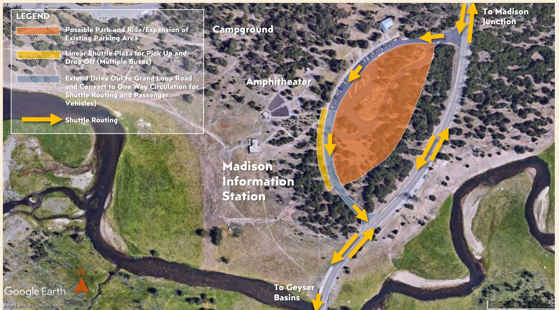
Figure 6.10—Conceptual Diagram for a Shuttle Terminal in the Madison Area of the Park
