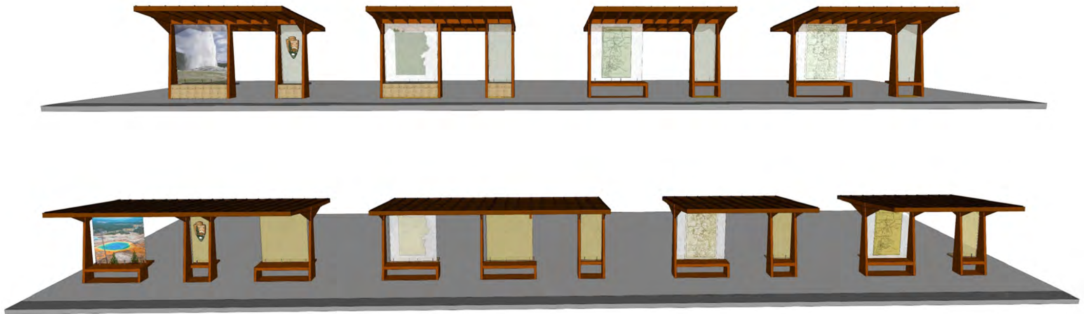
Figure 7.18—Kit of Parts Shelter Configurations—Shelters Can Be Expanded with Different Spatial Dimensions between Columns (Source: Roberts and Shelby, 2021)
