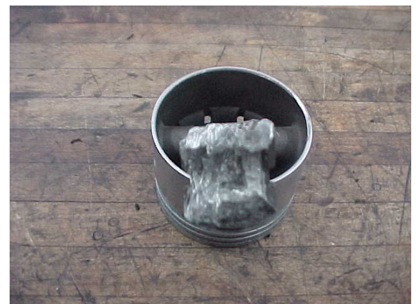
Scored crankpin bearing from insufficient lubrication.
