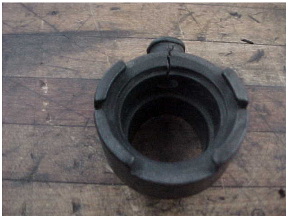
Cracked air cleaner grommet allows abrasive grit into engine.
