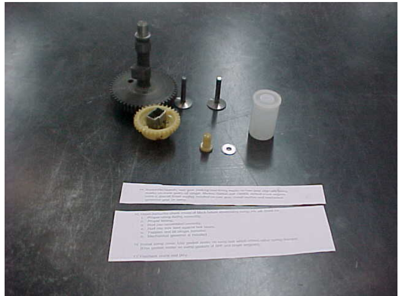
Cam gear, mechanical governor, and tappets
