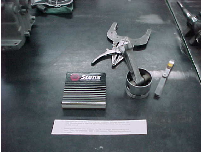
Parts and tools for installing rings and measuring ring land clearance.
