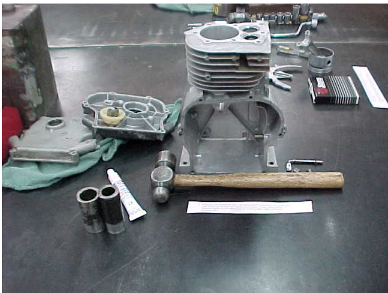
Tools for installing oil seals (oil seal drivers).
