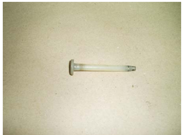
Fuel Tube-1 on Pulsa-Jet Carb.; 2 on Vacu-Jet Carb.
