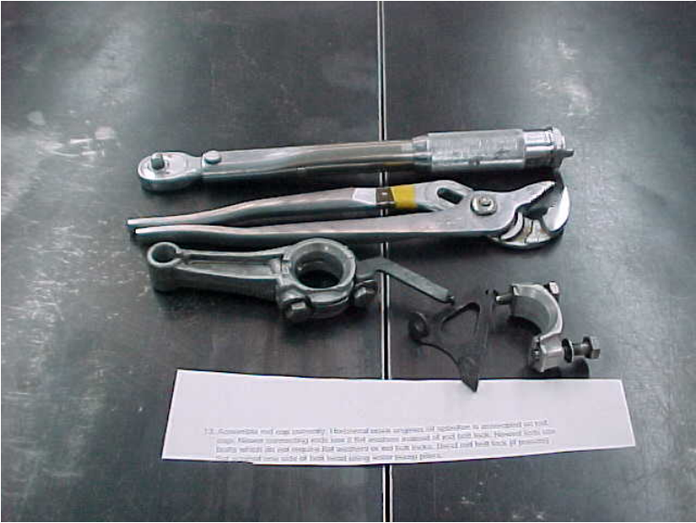
Tools and parts for assembling rod, rod bolt lock, and oil dipper
