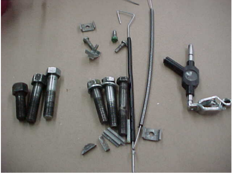
Speed control cables, speed control cable clamps and bolts, bolts and keys for flywheel weight, spark tester.
