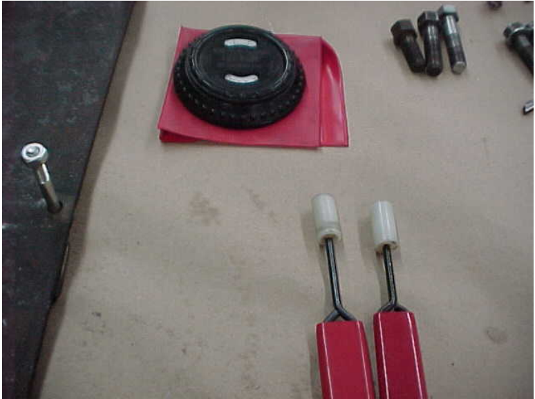
Briggs & Stratton carburetor screwdrivers have a plastic sleeve over them to keep the screwdriver on the screw while the engine is running. Vibration tachometer also shown.
