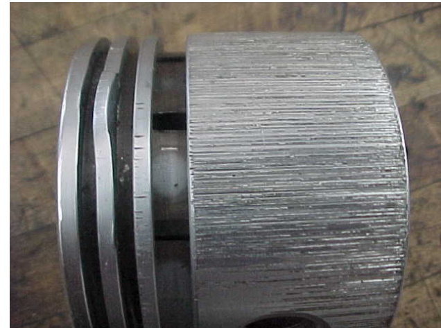
Worn piston from abrasive grit
