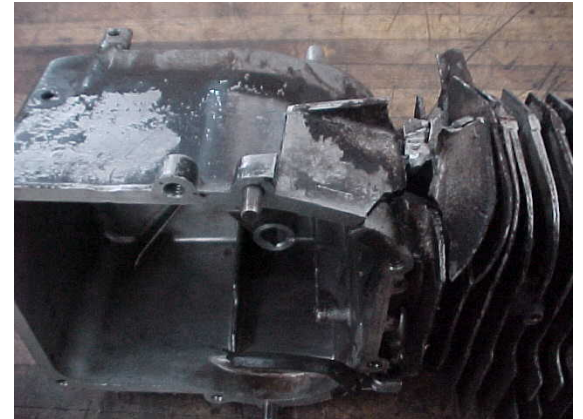
Broken block from broken connecting rod
