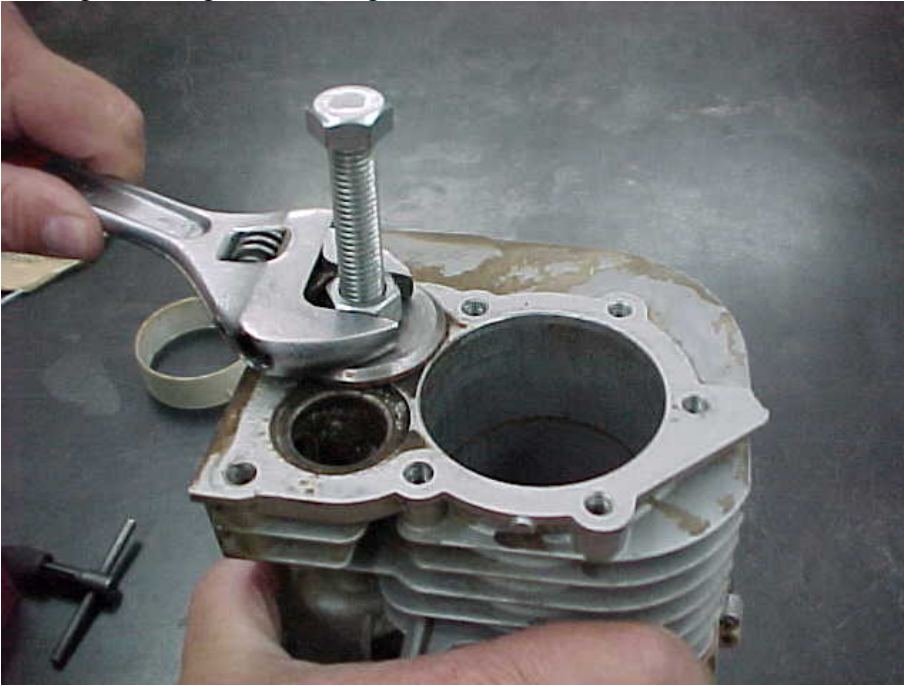
Valve guide bushing puller with old guide bushing on the end
