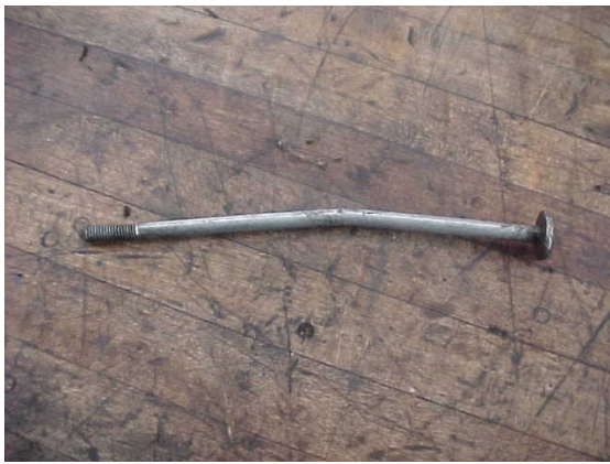
Bent air cleaner screw allows abrasive grit to enter engine
