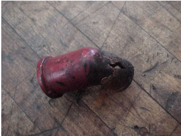
Cracked breather grommet allows abrasive grit into engine.
