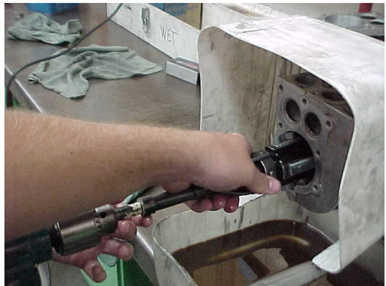
Over sizing a cylinder-tightening the hones, buckets cut to catch oil.
