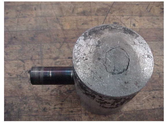
Discolored piston pin and damaged piston caused from overheating
