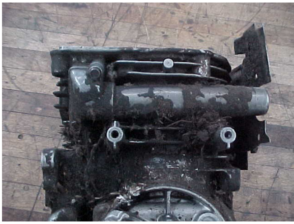
Clogged Cooling Fins
