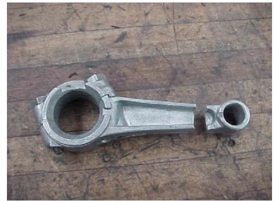
Broken connecting rod near piston pin from over speeding
