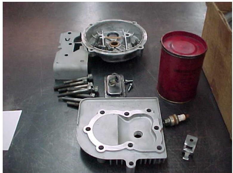
Head, head bolts, head shield, breather, graphite grease, spark plug, and kill switch.
