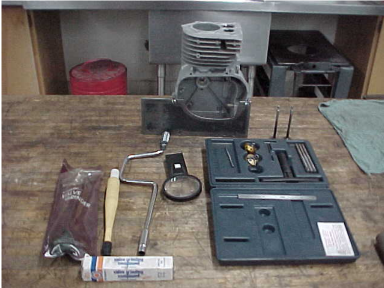
Valve seat cutter kit, valve lapping compound, engine block with vise mounting plate.
