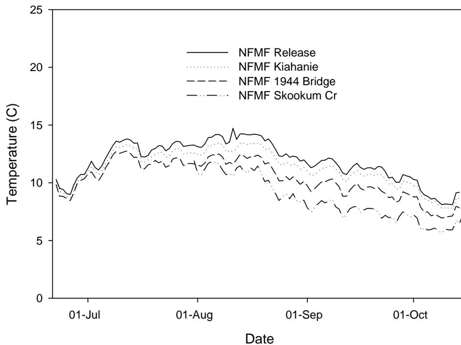
Figure 14. Daily mean water temperatures in 2012 at four sites in the North Fork Middle Fork Willamette River. The loggers represent a progression upstream from the release site (rkm 557.9) to Skookum Creek (rkm 585.9). Data gaps at the release site resulted from lost/stolen loggers.
