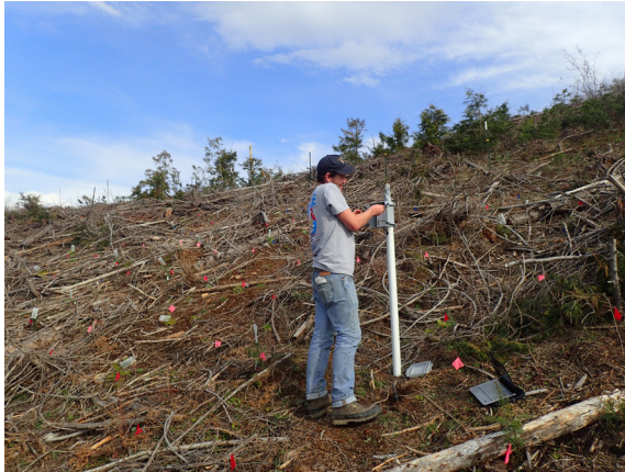
Figure 3. Soil moisture and temperature sensors were installed in each of the 9 blocks across the 3 sites
