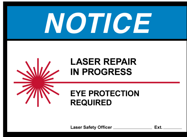
Figure 3.1: Example “Notice” sign for designating temporary laser controlled areas
