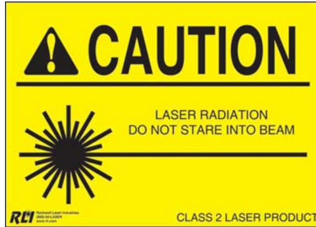
Figure 3.2: Example “Caution” sign for laser areas with class 2 or 2M lasers (for class 2, as shown)
