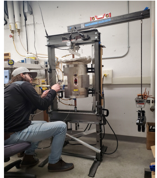
Tony DeSantis, MS student, checks the alignment and placement of an extensometer positioned within the creep furnace.
