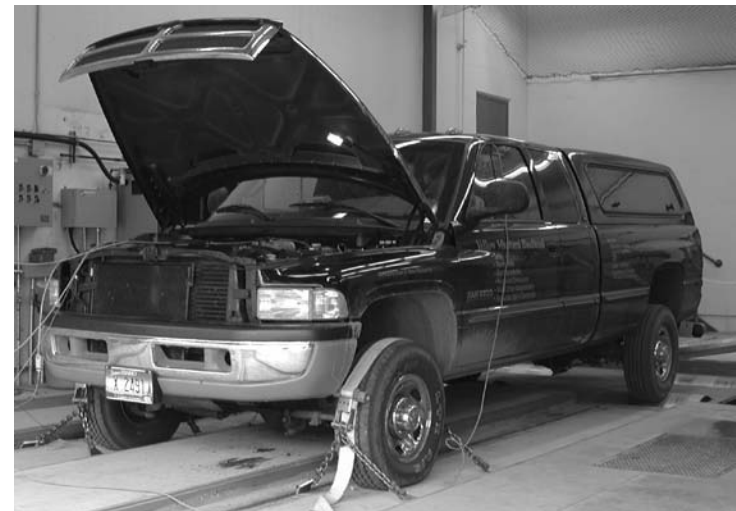
The Biodiesel Dodge pickup undergoes testing on chassis dynamometer.
