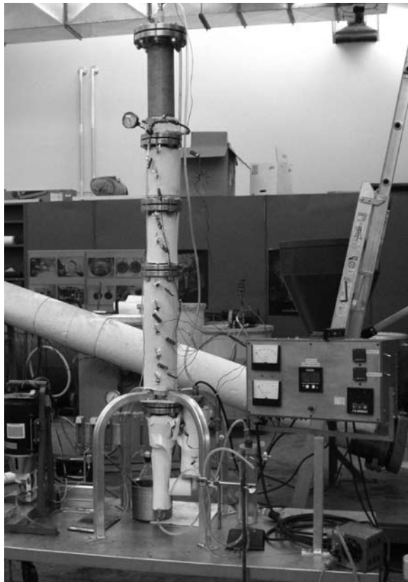
Set-up of the reactive distillation reactor for biodiesel preparation
