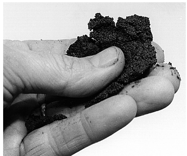
Fig. 9. A sandy loam textured soil, with 73 percent sand, 23 percent silt, and 4 percent clay, forms only a short, easily broken ribbon when squeezed between the thumb and fingers.
