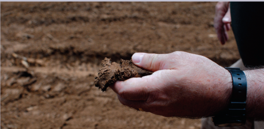
Using a soil ribbon to determine soil texture.
