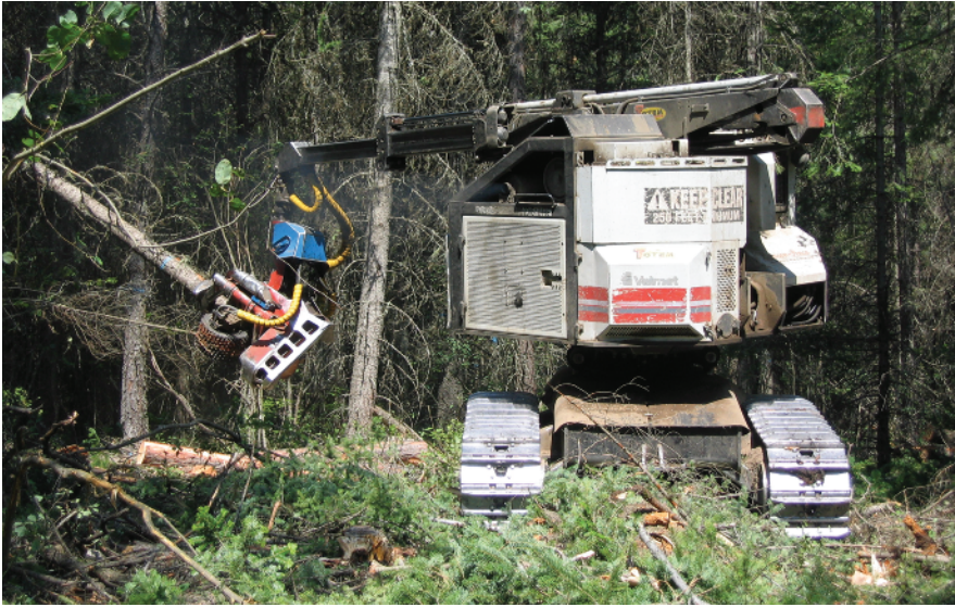
Feller-bunchers fell, limb, and cut logs to length at the harvest location.
