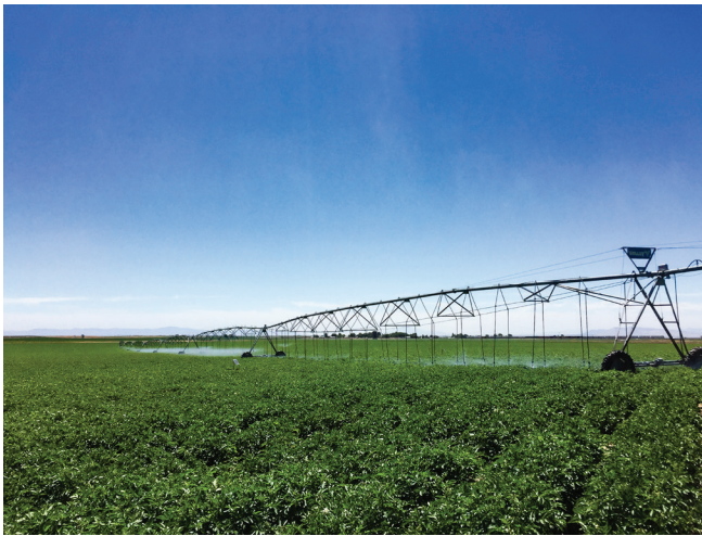
Figure 1. Adjacent spans of LESA (right) and MESA (left) in a potato field in Rupert, Idaho (Photo by Xi Liang).
