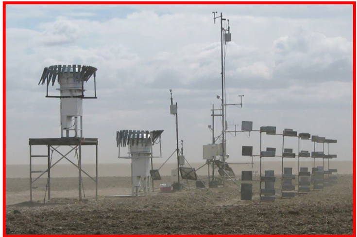
Figure 1. An array of dust emission recording instruments were installed on both the leeward and windward sides of 160-acre summer fallow fields in Adams County over eight years to quantify soil and carbon loss during wind storms.
