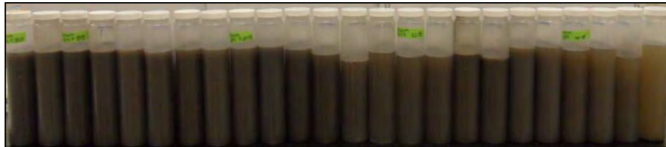
Water samples collected from Fourmile Creek upstream (top) and downstream (bottom) of the Fourmile Canyon fire during and after a thunderstorm on July 13, 2011. The downstream samples showed a substantial increase in turbidity (suspended material). (Photo by Sheila Murphy, USGS)
