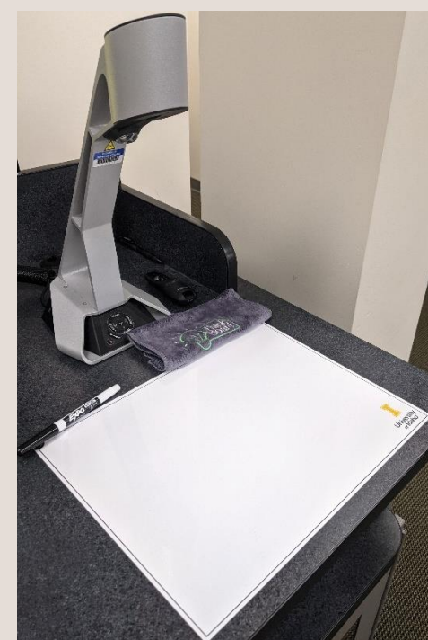
ThinkBoard dry erase film at every lectern to make use of the doc cam more convenient.
